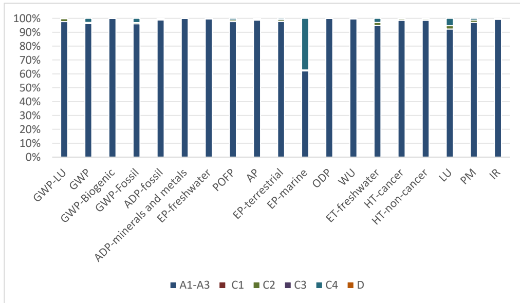
Figure 4. Ceiling Panels (Solid), Ceiling Tiles (Solid), Step Baffle, Fan Baffle, Solid Wall Panel - FilaSorb each stage contribution to LCA results
