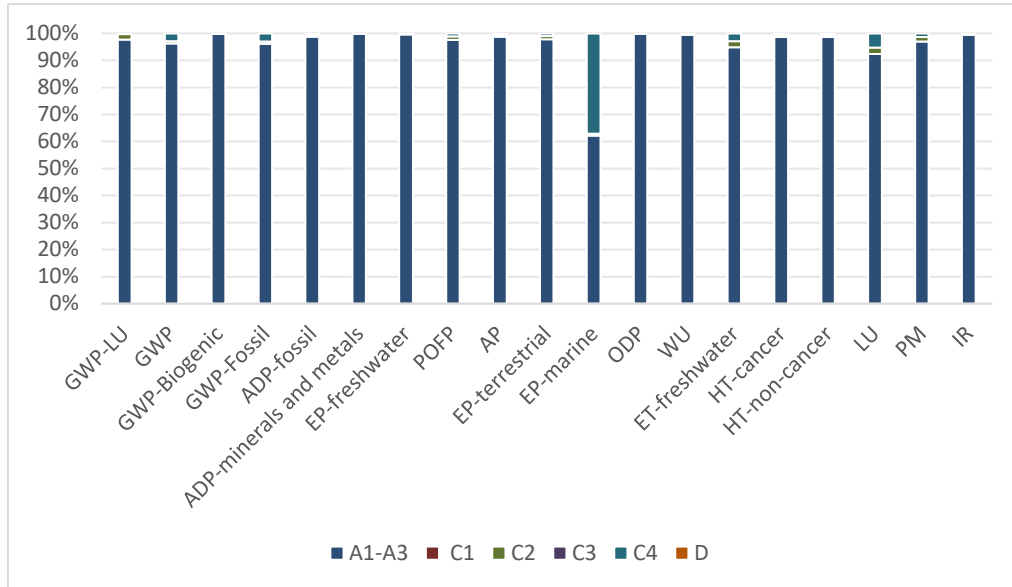
Figure 3. Arc Baffle, Ripple Baffle, Wing Baffle, Fracture Panel each stage contribution to LCA results
